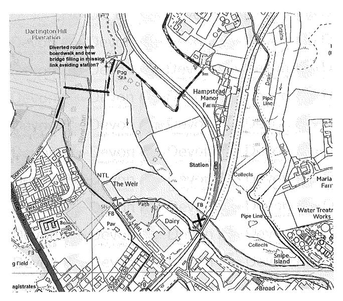
The exact position for the bridge is not determined but with a certain amount of sensible planning the bridge would be around this point with the aim of disrupting nature as little as possible yet providing a sensible solution to the impasse.
