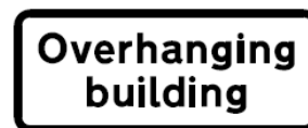
May be used only in combination with diagram 530A. A distance, an arrow pointing to the left or right or both may be added. "building" may be varied to "buildings" or to "structure"
