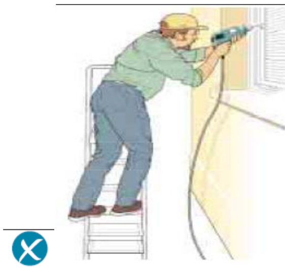
Incorrect – steps side on to work activity
